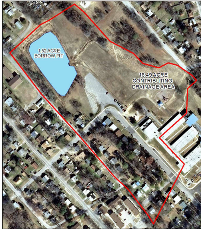
Figure 22. Existing borrow pit contributing drainage area (CDA). The borrow pit is presently 100% effective at water quality treatment of the 16.5-acre CDA.
